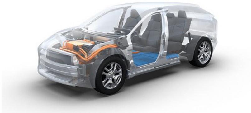
**Image: A BEV-dedicated platform Toyota and Subaru will jointly develop**
